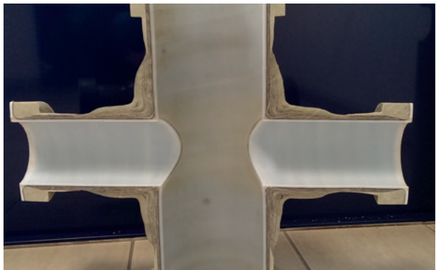
KERAVERIN® PTFE-M crosspiece after temperature change stress tests –50°C/+100°C
